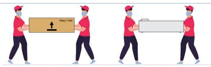
(1) A single package is approximately 50 kg. It is recommended to be moved by two persons. Keep the product level and upward during movement.
